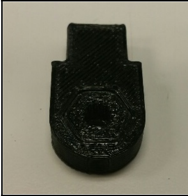
Figure 2.5: Gear Insert inside Bottom Motor Attachment
